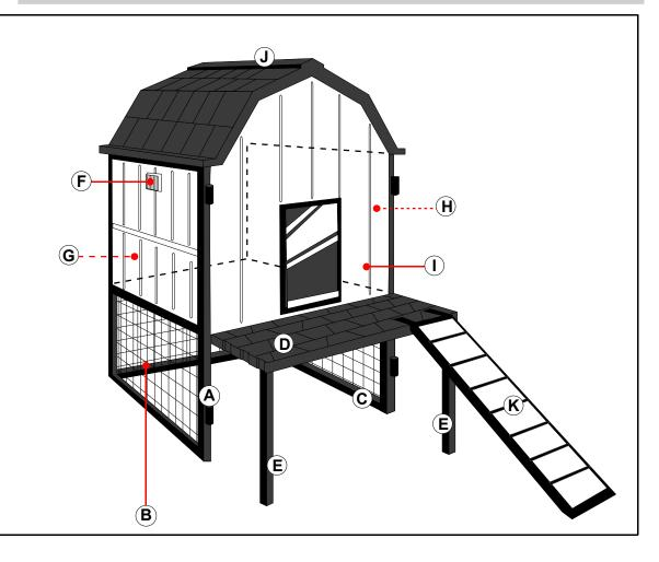
Connect the sides of parts A and C so that they form an angle of 90 degrees, insert the metal hinge center in the hinge hole provided. Do the same thing between parts B and C so that they form like the letter U.
